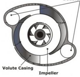
This figure show how the thrust is balanced by the Twin-Volute with 180 degrees opposite discharge outlets.
